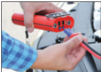
Once it Starts, Disconnect Clamps from Weego 44
