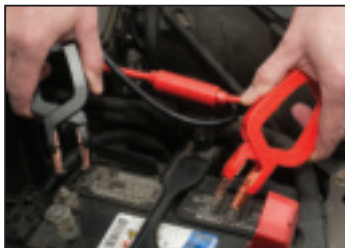
Detach Clamps From Battery
