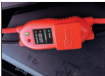
When You Have FLASHING GREEN LIGHT On Your Smart Box, Start Your Engine
